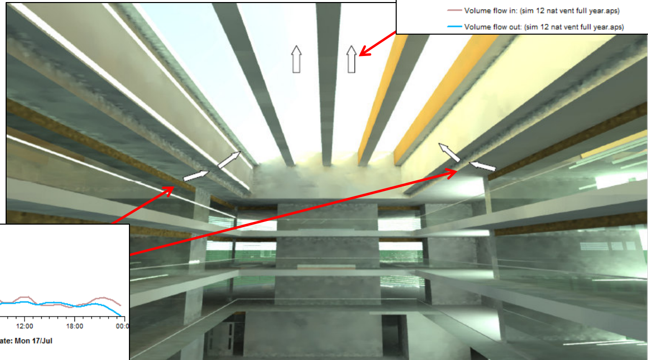
Natural Ventilation – Typical Airflow Through Atrium
