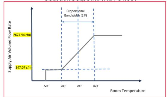
Figure 3: Controller 3: Zone VAV Cooling airflow Control (IP Units)
