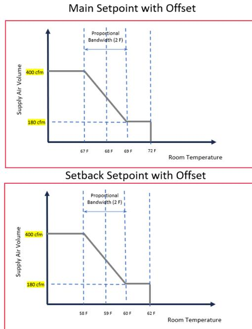
Figure 6: Controller 4: Zone VAV Heating airflow control
