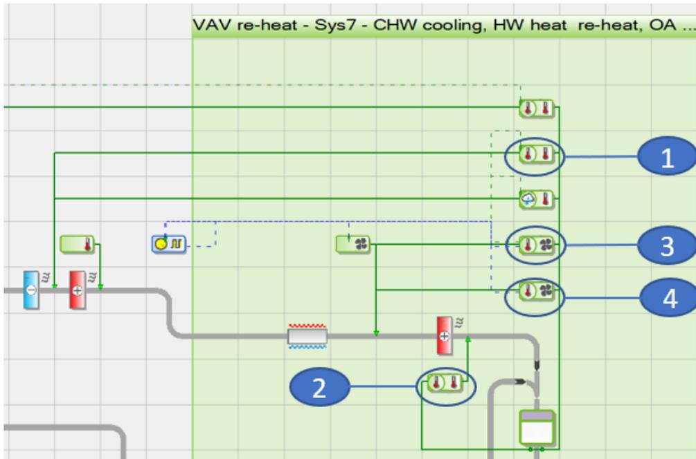
Figure 2: Typical VAV controllers in ApacheHVAC
