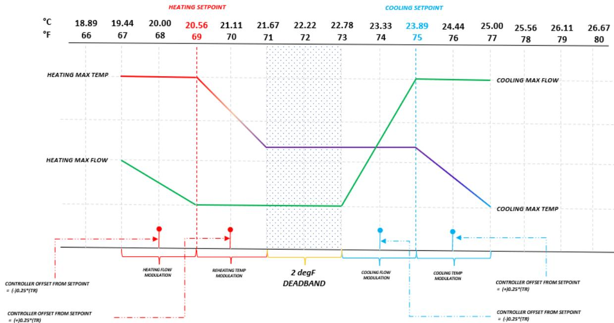
Figure 1: Typical VAV Operation cooling setpoint of 75 °F (23.89 °C) and heating setpoint of 69 °F (26.56 °C)
