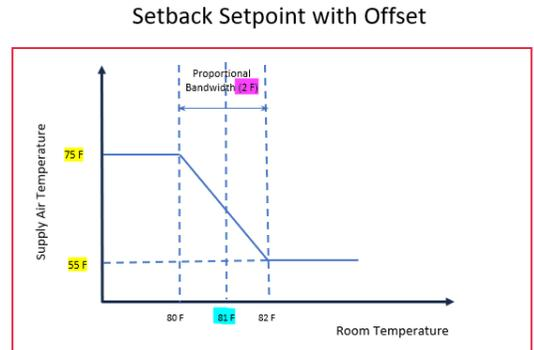
Figure 4: Controller 1: Cooling Coil Supply Air Temperature reset per zone demand (IP units)
