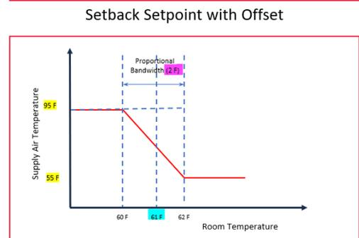
Figure 5: Controller 2: Zone Reheat Coil Supply Air Temperature reset
